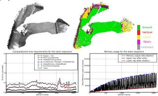
Fig. 2. Top: a snapshot of the point cloud data and semantic model for the stairs data set; bottom: computational time and memory usage requirements per useful stereo frame.
