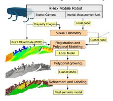
Fig. 1. The overall system architecture. obtained on the stairs dataset, together with its computational properties.
