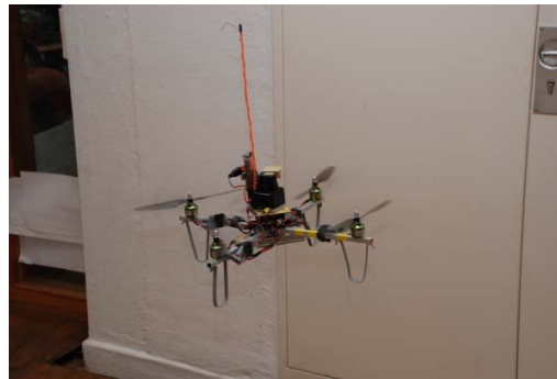
Fig. 24 Our quadrotor(left): 1) Mikrokopter platform, 2) Hokuyo laser range finder, 3) XSens IMU, 4) Gumstix computer. Right: Our System during a mission.
