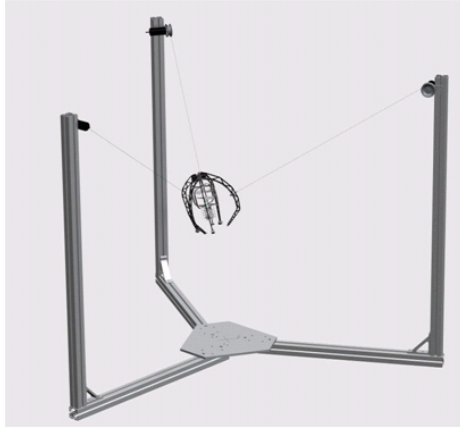
Fig. 4 The muFly vehicle test-bench. The central structure is supported by 3, actively controlled lines.
