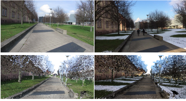
Fig. 5. Top: images from the Canon camera (left) and iPhone (right) datasets captured on the Freiburg campus. Notice the different weather conditions. Bottom: Post-colored 3D LiDAR map from a similar perspective.
