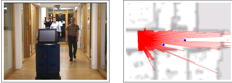
Fig. 3. Typical scene with two persons walking along the corridor (left image) and corresponding estimate of the laser-based people tracking system (right image).
