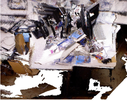
Fig. 3. Using only stepwise tracking leads to undesired results due to the accumulated drift (a). After graph optimization with 5 iterations of g^2o , an excellent alignment of most point clouds is achieved (b). Individual clouds are still slightly misaligned. Through integration of the free-space information these artefact are greatly diminished after computation of occupancy probabilities (c).
