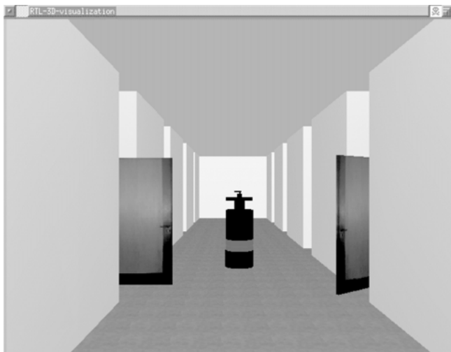
Figure 2: Rhino detecting the state of two doors with its laser range-finder (upper image). The estimated states of the doors are depicted in black. The resulting 3D-visualization is shown in the lower image.
