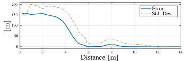
Fig. 2: Mean particle position error (solid line) and particle position standard deviation (dashed line) over traveled distance, for the NDVI map based particle filter solving the global localization problem. The particle filter requires the robot to travel a certain distance before it is able to correlate measurements with the map. After that, it quickly converges to the true position, while maintaining multiple possible solutions due to map symmetries.
