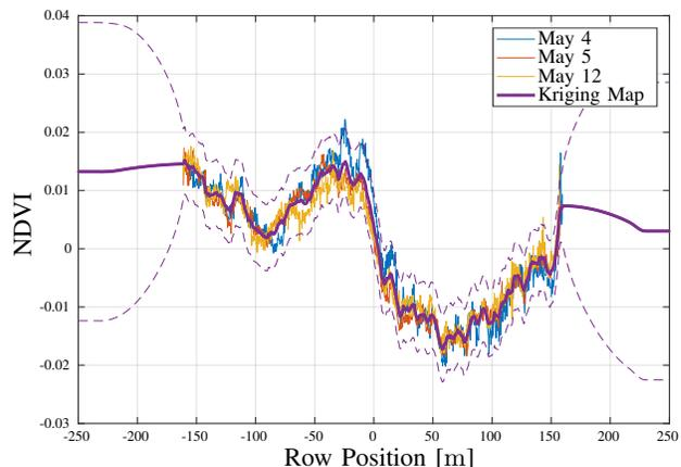
Fig. 1: 1-D mean NDVI map obtained via Kriging (purple line with confidence interval indicated by the dashed lines) along with the three raw measurement series (from May 4, 5 and 12, 2016) used for map construction.
