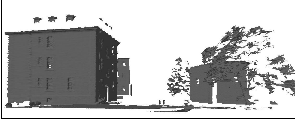
Figure 2: Polygonal model obtained after registering two scans using our probabilistic method.
