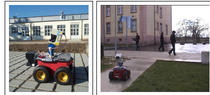
Figure 7: Pioneer 2 AT robot used for 3d mapping (left) and typical situation in which people walk through the scene during mapping (right).
