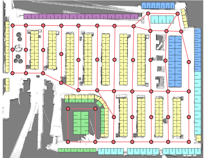
Fig. 1: Example map of a real supermarket environment. In our approach, maps contain shelf locations, shelf types, and product locations. The underlying structure is a graph. The task of the robot is to efficiently find a target product and to guide the search by utilizing the local information given by its current location and the products in its direct vicinity.
