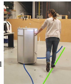
Fig. 1. Whole-body tactile sensory concept and robot prototype reacting to an external interaction force.
