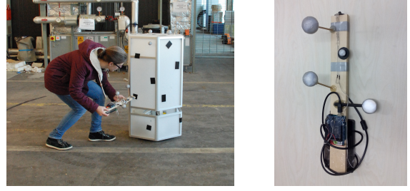
Fig. 3. Force stick used to exert and measure external forces on the robot shell. The optical markers are used to determine the 6D pose of the stick with respect to the robot.
