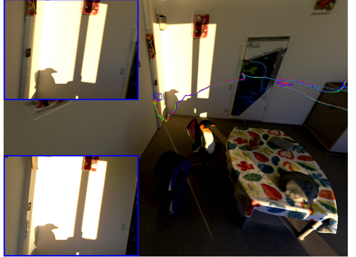
Fig. 1: 3D model of a scene used for camera tracking. We estimate the outdoor illumination using the current camera image shown in the left bottom corner. The image in the left top corner is rendered from the model with the same camera view.
