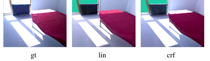
Fig. 5: Comparison of illumination scales estimated with the linear-least-squares (lin) and CRF-based error function. The lin approach tends to underestimate the brightness in over-exposed image regions, as seen in the sun-lit part of the table. The CRF method, in contrast, is significantly closer to the ground truth (gt).
