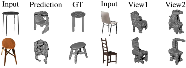
Fig. 7: Certain failure cases. On the top left example the network predicts an approximate shape of the round chair, but fails to remove the mean shape. For the bottom left case, the network fails to predict a consistent shape. On the right, it reconstructs shapes which only fit the input view and look incorrect from unobserved viewpoints.
