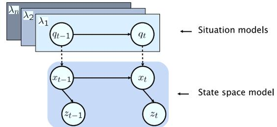
Fig. 1. Schematic representation of the proposed framework for situation modeling and recognition. Each situation type is described by an individual HMM  $\lambda_i$ . A situation instance exists as long as the corresponding HMM recognizes the state sequence being generated.
