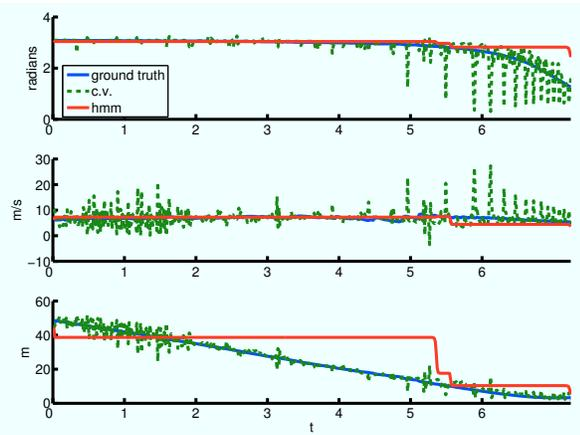
Fig. 8. 1-second prediction for a sequence corresponding to a passing vehicle according to a constant velocity model (c.v.) and our learned HMM-based *passing* situation model (hmm).
