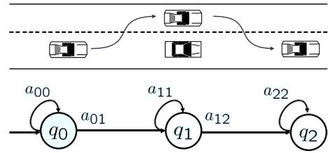
Fig. 2. A *passing* maneuver, in which the reference vehicle (square car in the middle) is being passed on its left hand side by another one. In this case, we divided the maneuver into three stages and, thus, used a 3-state HMM over abstract world states as a model (bottom).
