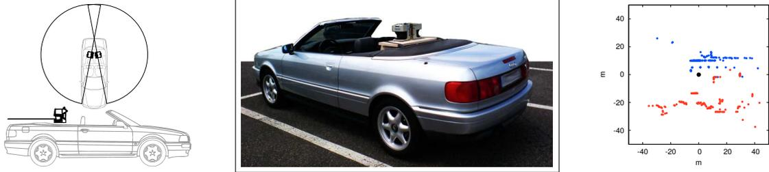
Fig. 5. Left: arrangement of two SICK laser range finders on a convertible (middle) used for gathering real data. Each laser has a field of view of 180 degrees and can detect objects as far as 80 meters with an angular resolution of 1 degree at 75Hz. The arrangement of the two lasers provided a 340 degree field of view (right).
