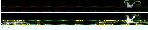
Fig. 6. Landmark configuration and uniqueness before and after placing the landmarks for the building 103 data set gathered with a real robot using a laser range scanner.
