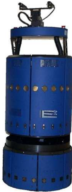
Figure 5.4: The image shows the robot used for the experiments, a B21r robot equipped with a SICK laser range finder and a camera system mounted on a pan/tilt unit.
