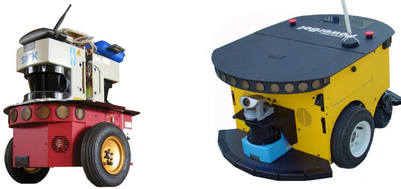
Figure 3.9: On the left, an ActivMedia Pioneer 2-DX8 equipped with two SICK laser range finders. On the right, a PowerBot robot equipped with a front laser.
