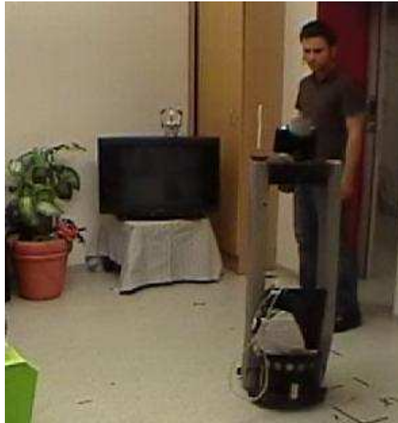
Figure 8.10: Following the order “go to the television”, the robots approaches the navigation node from where it saw the television the last time.
