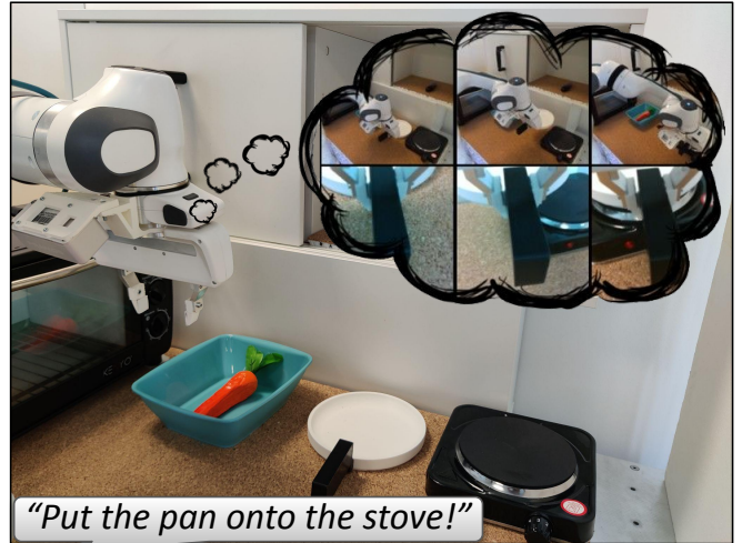
Fig. 1: LUMOS learns a general-purpose language-conditioned visuomotor policy within the latent space of a learned world model. By optimizing an intrinsic reward to match expert performance, it recovers from its own mistakes across multiple time steps and reduces covariate shift. As a result, LUMOS can handle complex, long-horizon robot tasks from abstract language instructions in real-world scenarios, without online learning or fine-tuning.
