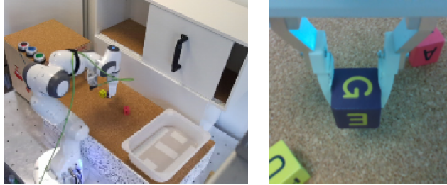
Figure 6. Visualization of the observations obtained in the real world environment. On the left we show the RGB image captured by the static camera. On the right we show the RGB image captured by the gripper camera.
