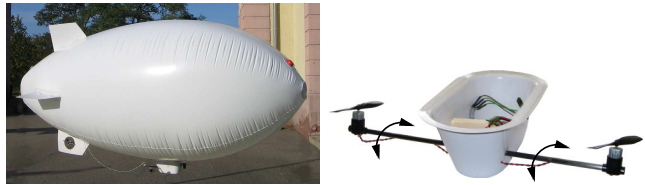
Fig. 1. Blimp used to evaluate our approach (left image). The right image shows the gondola with two rotors for pitch and thrust control. They can be rotated by 180 degrees.
