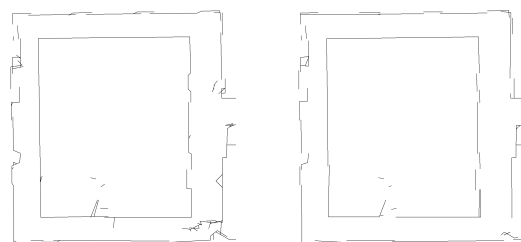
Fig. 6. Fraction of the line maps for the Sieg-Hall data set generated by the incremental (left) and offline (right) approach.
