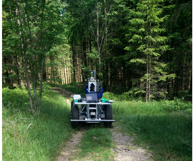
Fig. 1: Our mobile robot VIONA while recording the forest dataset.
