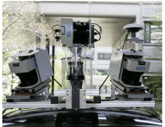
Fig. 4. Sensors mounted on the roof
