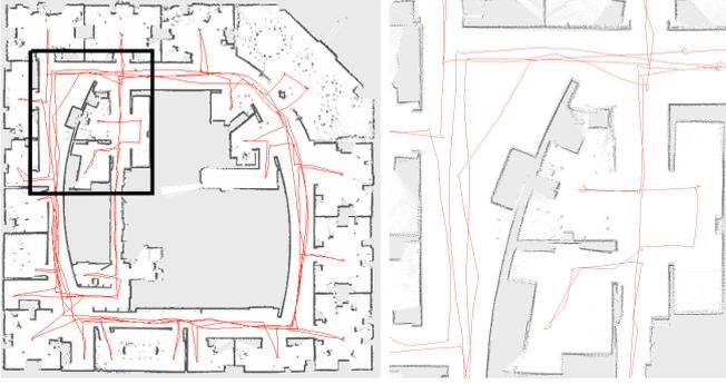
Fig. 3. The Intel Research Lab. The robot starts in the upper part of the circular corridor, and runs several times around the loop, before entering the rooms. The left image depicts the resulting map generated with 15 particles. The right image shows a cut-out with 1 cm grid resolution to illustrate the accuracy of the map in the loop closure point.
