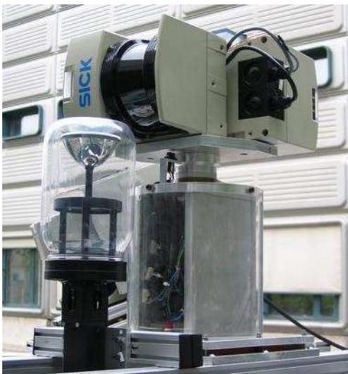
Fig. 5. Rotating scanner and omnidirectional camera
