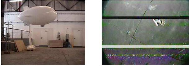
Fig. 5. The left image depicts our blimp and the right one example images received via the analog video transmission link.
