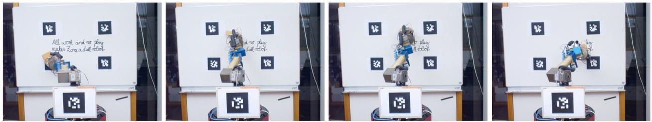
Fig. 8. The reproduction of the board cleaning task by our robot. It imitates the zig-zag movement for cleaning the board with the sponge. Note that the learned task representation allows for cleaning differently sized surfaces based on the markers.
