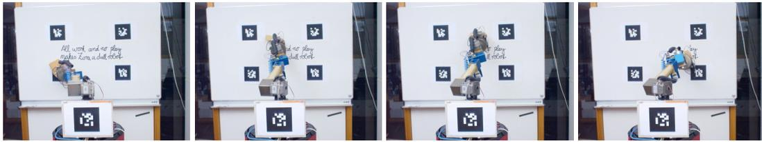
Figure 6.9: The reproduction of the board cleaning task by our robot. It imitates the zig-zag movement for cleaning the board with the sponge. Note that the learned task representation allows for cleaning differently sized surfaces based on the markers.
