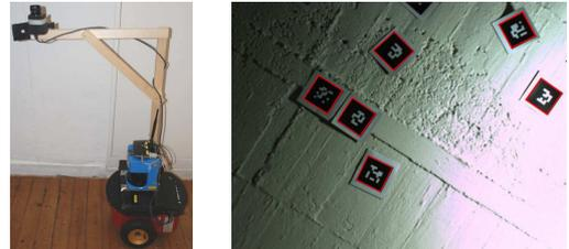
Fig. 4. Pioneer 2-DX8 robot with upward-looking camera and SICK laser range scanner (left) and detected visual landmarks on the ceiling (right).
