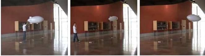
Fig. 8. A person pushes the blimp away. The blimp is able to localize itself and navigate back using the map shown in Figure 7 (see video material).
