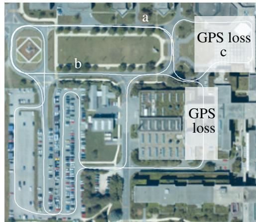
Figure 6.5: Overlay of the estimated trajectory and the ortho-photo of the EPFL campus. The zones where the GPS was not available are highlighted. The total traveled distance is around 2300m. The labels (a), (b), and (c) identify areas where GPS errors occurred but which did not cause pose estimation failures due to the multi-sensor data fusion.
