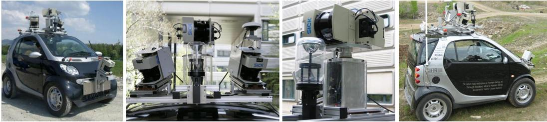
Figure 6.4: Our computer-controlled Smart car and the sensor setup mounted on the roof of the car. The right image shows our car during the first European Landrover Trials (ELROB).
