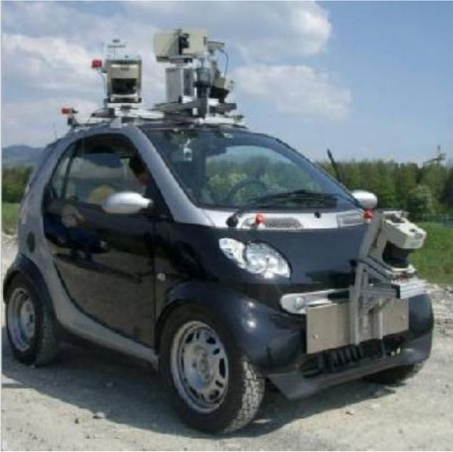
Fig. 1. Our autonomous Smart car platform. There are three fixed laser range finders mounted on the front of the vehicle and on the sides of the roof, and two spinning laser range finders mounted together on the center of the roof. Inside the vehicle, mounted behind the windshield, is an automotive camera used for lane detection.
