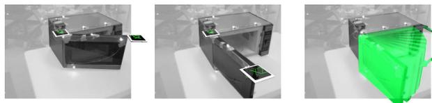
Figure 1: Left and middle: examples for observations of a moving door of a microwave oven. Right: visualization of the kinematic model of the door learned by our approach.
