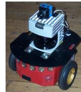
**Fig. 3.** Wheeled robot equipped with a perspective camera.
