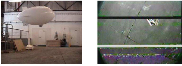
Fig. 5. The left image depicts our blimp and the right one example images received via the analog video transmission link.
