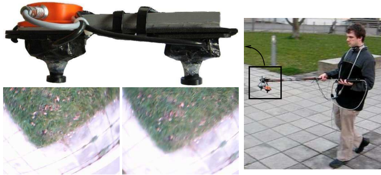
Fig. 1. Top Left: the sensors used for testing our approach. We assembled two cheap USB webcams as a stereo pair and combined it with a Xsens MTi inertial measurement unit. Bottom Left: a typical stereo image used for constructing the map. Note the significant motion blur affecting the image. Right: the procedure for acquiring the data. We mounted the sensors with the cameras looking downwards on a stick and we then walked around the campus.
