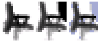
Fig. 4. Range image as it should look like according to the model (left) and actual part of the scene range image (middle). The black part on the top right of the image is clutter in front of the object. The right image shows the overlay of the other two images. The parts that are too different are marked in blue.
