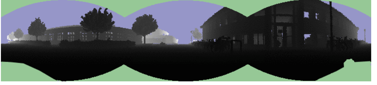
Figure 7.2: Example range image from the FreiburgCampus360_3D dataset (see Section 7.2.1 for details on the dataset). The image pixel positions represent the spherical coordinates of the points. The gray values represent the measured ranges. Blue points are maximum range readings and green points are unknown space.
