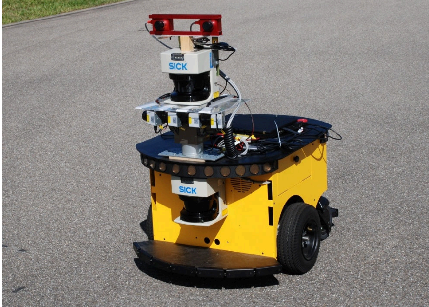
Figure 8.6: The robot we used for our experiments. The top SICK laser range finder mounted on a pan-tilt-unit was used to acquire the needed 3D scans. (Source: [73])
