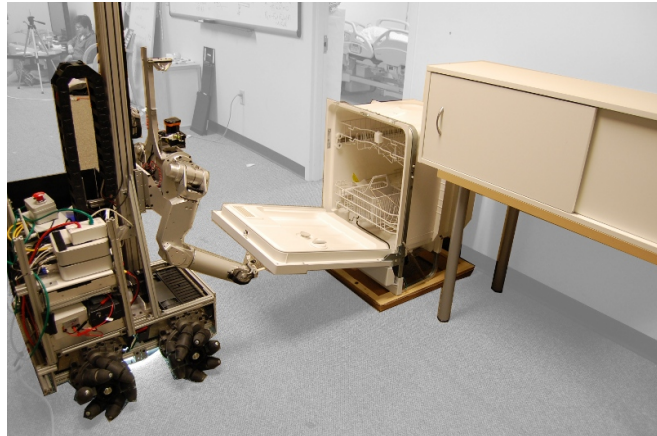
Fig. 1. Our service robot successfully opens various articulated objects (here: a dishwasher) by generating equilibrium control points from the kinematic model that it learns online from its end effector trajectory.
