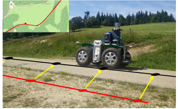
Fig. 1. Our approach addresses robot navigation in outer-urban environments and aims to match a path given from OpenStreetMap (red) to the part in the sensor data that may most likely corresponds to the street (black). It is particularly designed to cope with map and GPS errors.
