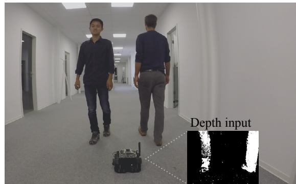
Fig. 1: A mobile robot navigating in a socially compliant manner in an indoor environment. Our approach tackles this scenario through raw depth images.
