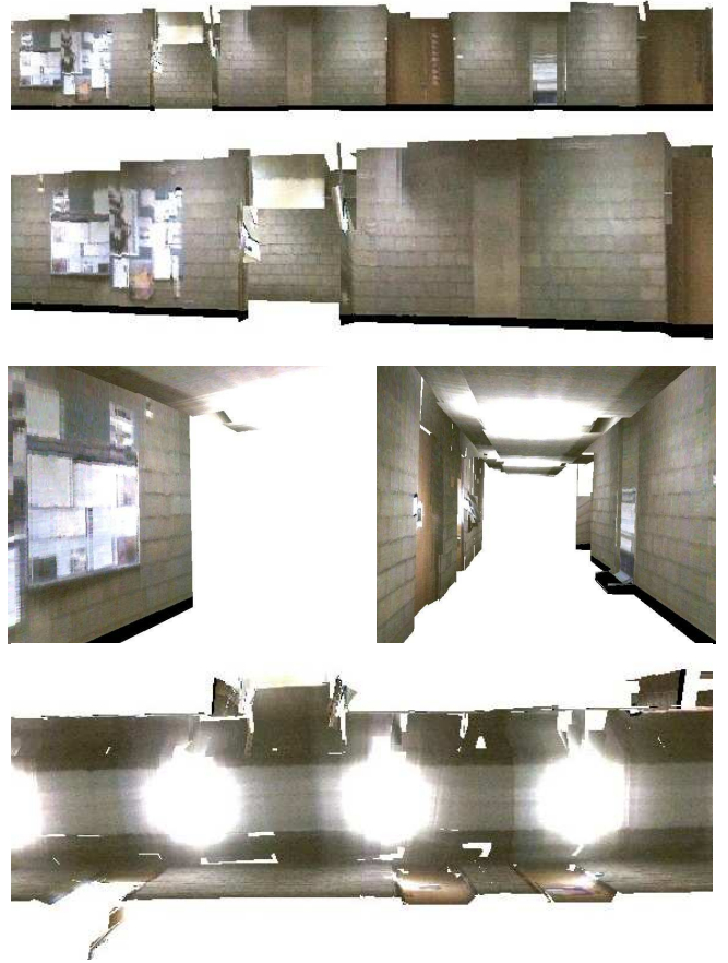
Fig. 8. Views of a compact 3D texture map built in real time with an autonomously exploring robot.
