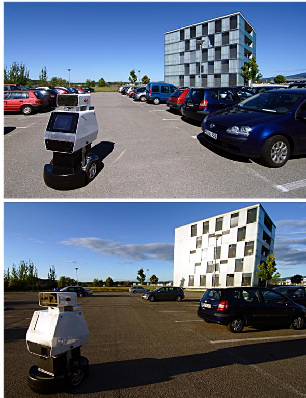
Fig. 1. A mobile robot with a horizontally scanning laser range finder navigating in a parking lot at noon (top) and at 6 pm (bottom). Note that despite being at the same spot in both cases, the perceived scans will be substantially different due to the changed number of parked cars.
