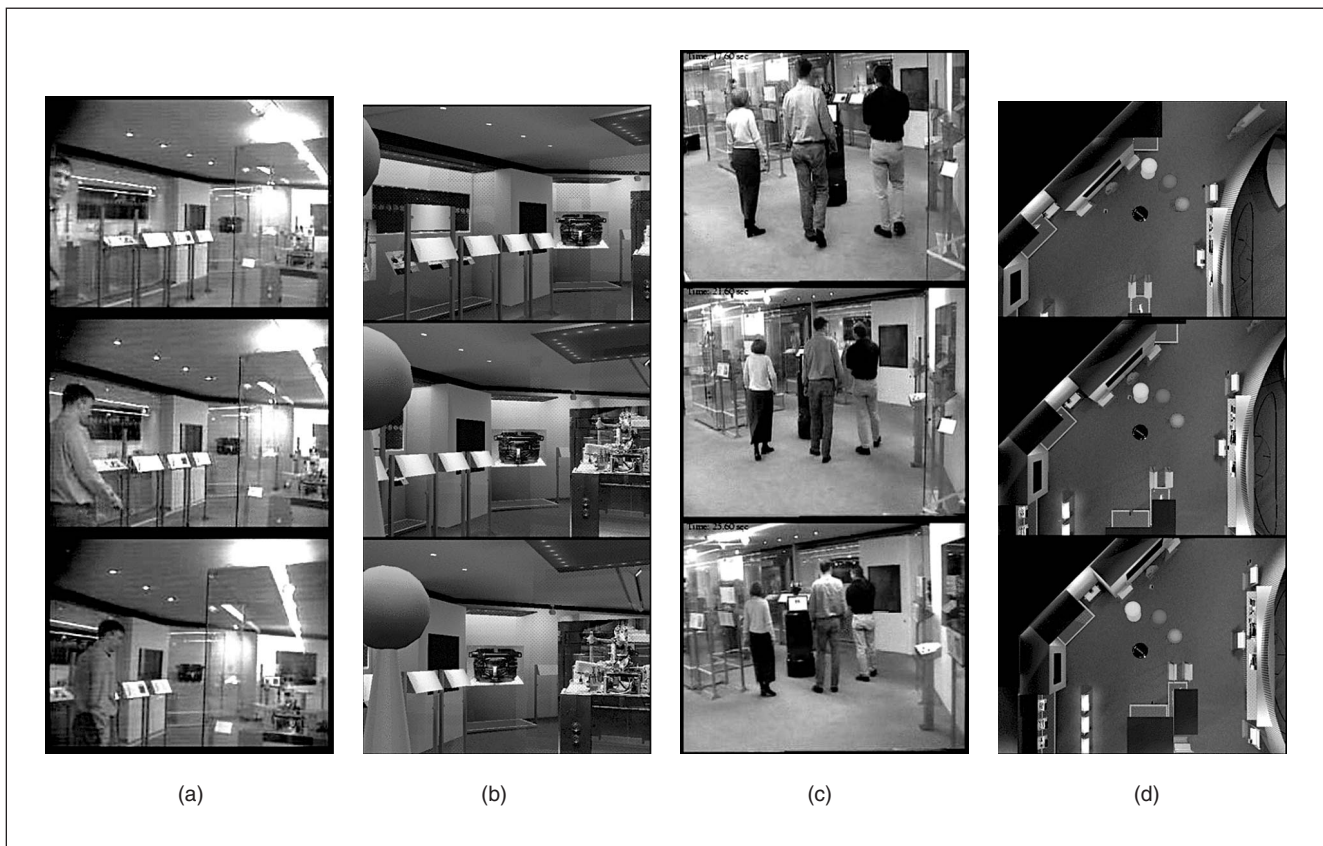
Figure 8. The enhanced 3-D visualization allows arbitrary viewpoints: (a) the real and (b) the virtual view through the robot's cameras and (c) the robot guiding three people through the museum and (d) a bird's eye view of the scene.
