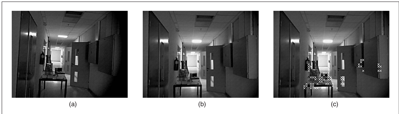
Figure 5. (a)–(b) Images acquired at successive points in time and (c) results of obstacle detection superimposed on the image shown in (b).
