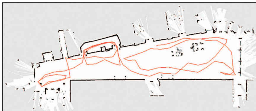
Figure 2. Map generated using our Rao-Blackwellized mapping algorithm. The size of the environment is 18 \times 51 m. The robot had to close several loops during the mapping process.
