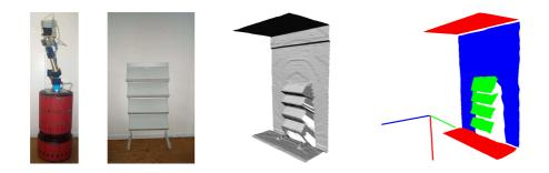
Fig. 4. Mobile robot Zora (left image), scene scanned by the robot (second image), resulting data (third image), and final model (right image).
