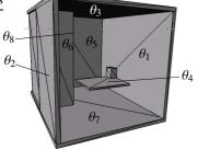
Fig. 6. Simulated 3d scene used to evaluate the quality of the resulting maps. On top of the horizontal plane is a small cube that introduces errors in the plane extraction.
