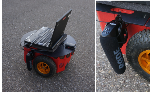
Fig. 3 The Pioneer P3-DX platform showing the shotgun microphone with the shock mount, mounted close to the wheel.
