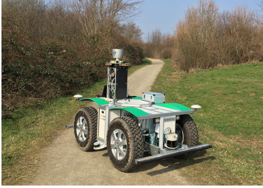
Fig. 3. The Viona autonomous mobile robot platform equipped with bumblebee stereo cameras and a modified dashcam with the NIR-cut filter removed for capturing RGB and NIR images respectively.
