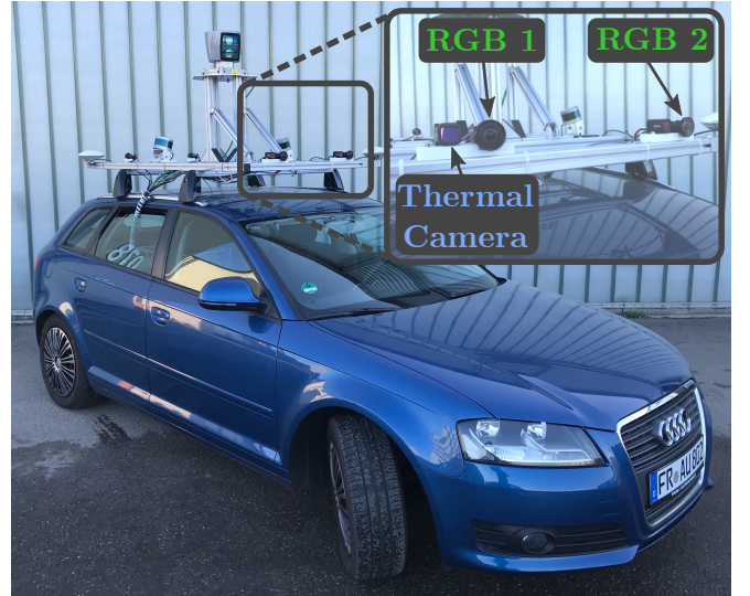
Fig. 3. Our stereo RGB and thermal camera rig mounted on our data collection vehicle.
