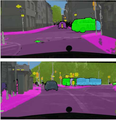
Fig. S-3. A limitation of our method is that occluded objects are separated into multiple instances.
