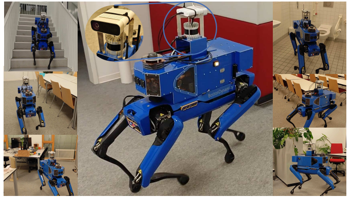
Fig. 9: Boston Dynamics Spot robot exploring a two-story office building with multiple types of rooms. The quadruped is equipped with an Azure Kinect RGB-D camera and a 3D LiDAR to collect RGB-D data and odometry.
