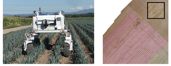
Fig. 6: Our agricultural robot, the BoniRob, on a leek field (left). The right side shows a georeferenced image of a sugar beet field overlaid with a crop row pattern (magenta) extracted from the image data.
