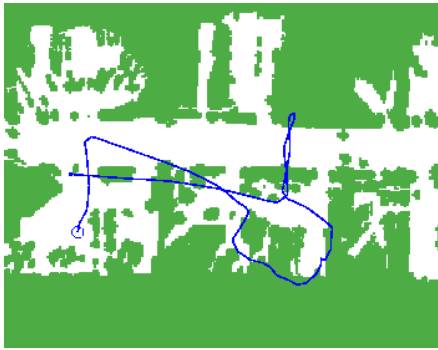
Fig. 9. Trajectory of the robot according to the odometry data.
