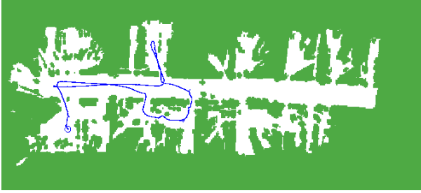
Fig. 8. Map of the office environment used to carry out the experiments and trajectory of the robot (ground truth). The size of the environment is 37 m times 14 m.
