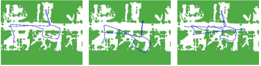
Fig. 4. Map of the office environment used to carry out the experiments and trajectory of the robot (ground truth) (left image). Trajectory of the robot according to the odometry data (center image). Positions of the robot estimated by our system during global localization (right image)
