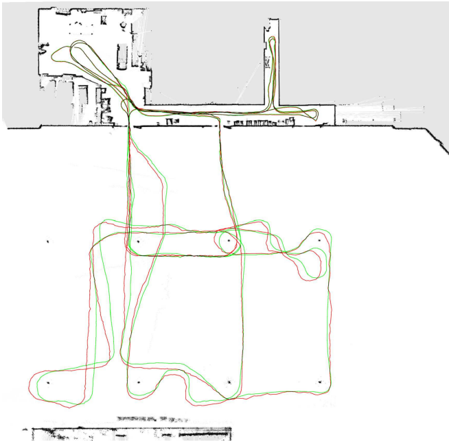
Fig. 7. Grid map of parking space and neighboring building 078 at Freiburg campus. The approximated robot trajectory is shown in red/dark gray, the result of our combined mapping approach is shown in green/light gray.
