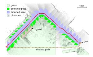
Figure 14: Autonomous navigation experiment. Although the shortest obstacle-free path from the start to the goal position led over grass, the robot reliably avoided the vegetated areas by using our vegetation classifier and traveled over the paved streets to reach its goal.
