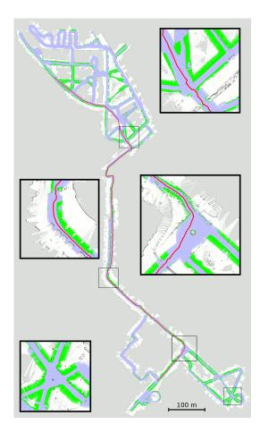
Figure 15: Autonomous navigation experiment. The robot planned a path on a map annotated by our approach. The robot autonomously traveled a distance of approximately 1,120 m. Each black rectangle shows a magnified view of a particular area of the environment.
