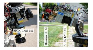
Figure 6: Sensors used in the evaluation.
