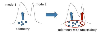
Sample from odometry first and the use this as the start point for scan matching
