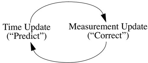
**Figure 4.1:** The ongoing discrete Kalman filter cycle. The *time update* projects the current state estimate ahead in time. The *measurement update* adjusts the projected estimate by an actual measurement at that time.
