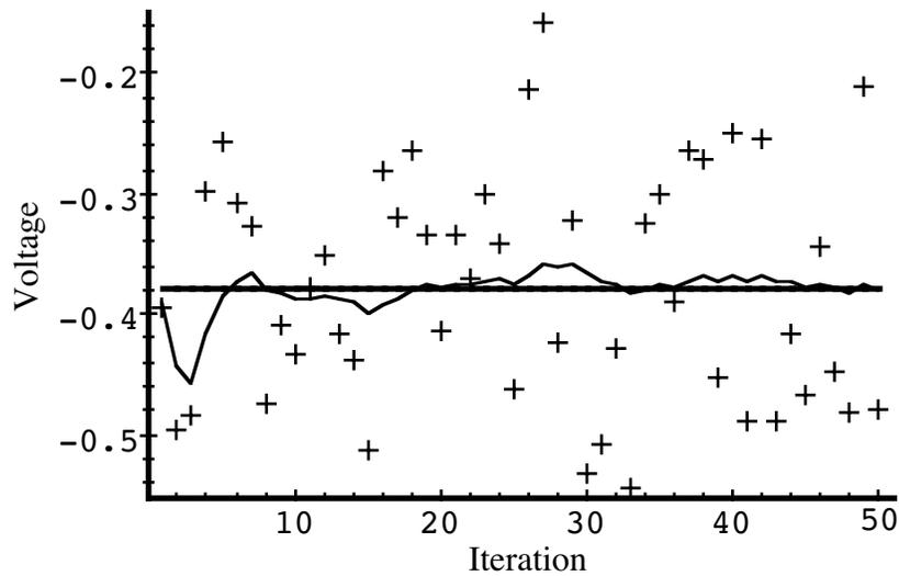
**Figure 4.4:** The first simulation:  $R = (0.1)^2 = 0.01$ . The true value of the random constant  $x = -0.37727$  is given by the solid line, the noisy measurements by the cross marks, and the filter estimate by the remaining curve.
