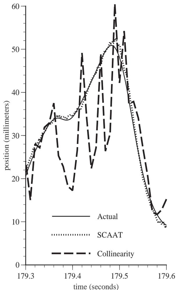
Figure 4: The upper plot depicts the entire 3 minutes of  $x$ -axis position data from user motion data set ‘a’ of sets ‘a’-‘f’. The lower plot shows a close-up of a short portion of the simulation. Collinearity here used  $N = 10$  beacons per observation, hence its lower estimate rate. On the other hand, notice that the SCAAT estimates and the actual (truth) data are almost indistinguishable.
