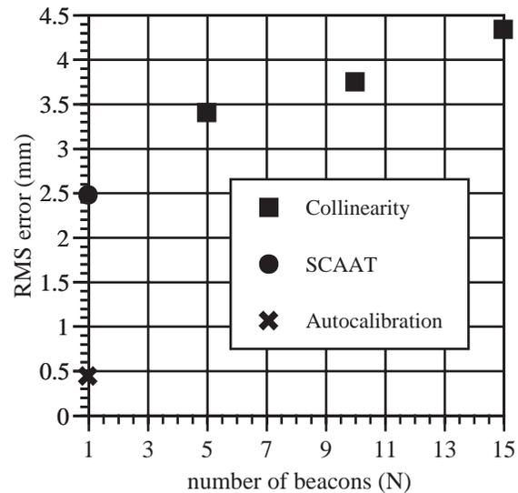
Figure 5: As the number of beacons  $N$  is reduced from 15 to 5, the Collinearity results improve slightly. (The Collinearity algorithm generally becomes unstable with  $N \leq 4$ .) The SCAAT results, with  $N = 1$  beacons, are better, and especially good once autocalibration is turned on.
