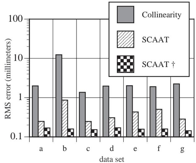
Figure 7: RMS error results for simulations of all seven real user motion data sets. The  $\dagger$  symbol indicates a second pass through the motion data set, this time using the already autocalibrated beacons.
