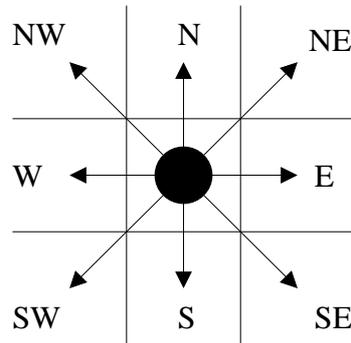
(b) Possible single-step movements of a robot in a simple grid world.
