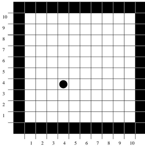
(a) Representation of the state space of a robot using an occupancy grid. Cells can be occupied (black-colored cells) or not (white-colored cells). The state  $x$  of the robot is specified by the cell it occupies.
