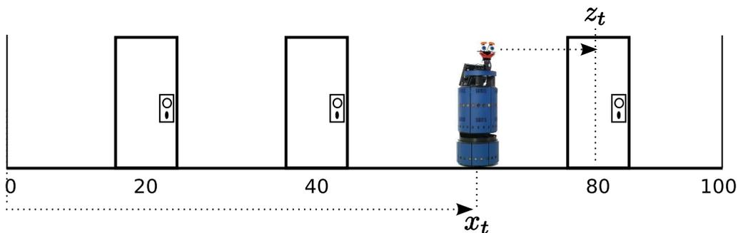
Figure 1: The state  $x_t$  of the robot corresponds to the distance of the robot to the start of the corridor. Each sensor measurement  $z_t$  is a single range reading that corresponds to the distance between the robot and the nearest door.
