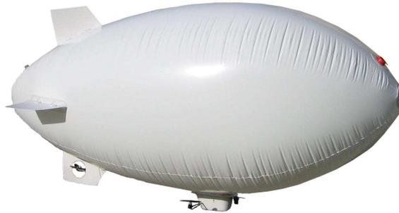
Figure 1: The blimp is equipped with downward-looking ultrasound sensor for measuring the vertical distance to the underlying obstacles.
