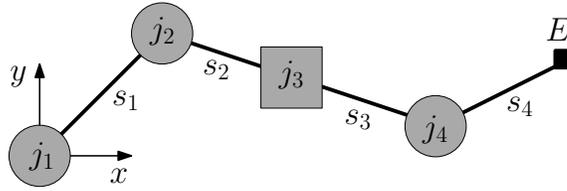
Figure 1: Manipulator with three rotational and one prismatic joint.
