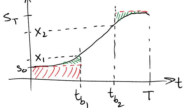
③  $x_1 - s_0 = v_0 t_{b_1} + \frac{1}{2} a_{\max} t_{b_1}^2$
